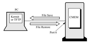
Figure 6-4. Saving/Restoring Vanguard 6520/6560 Configurations Using Kermit or TFTP
