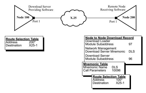
Figure 4-3. Critical Crossloading Parameters
