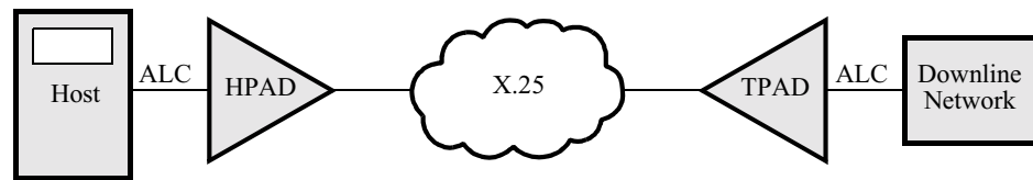
Figure 1. Combined HPAD TPAD Operation
