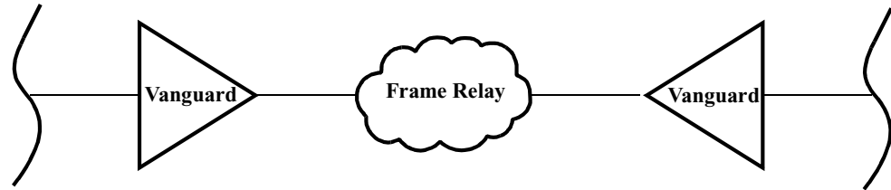
Figure 3. Ethernet Bridge Example
