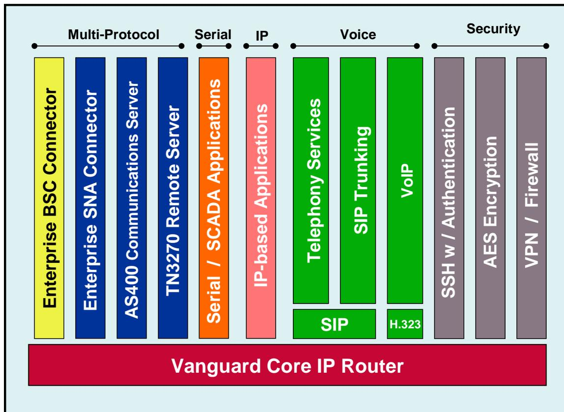
Enterprise BSC Connector is one of the many applications offered in the ApplicationsWare suite that operate on the Vanguard IP Router base platform. All applications can be run across a single wide area network environment.
