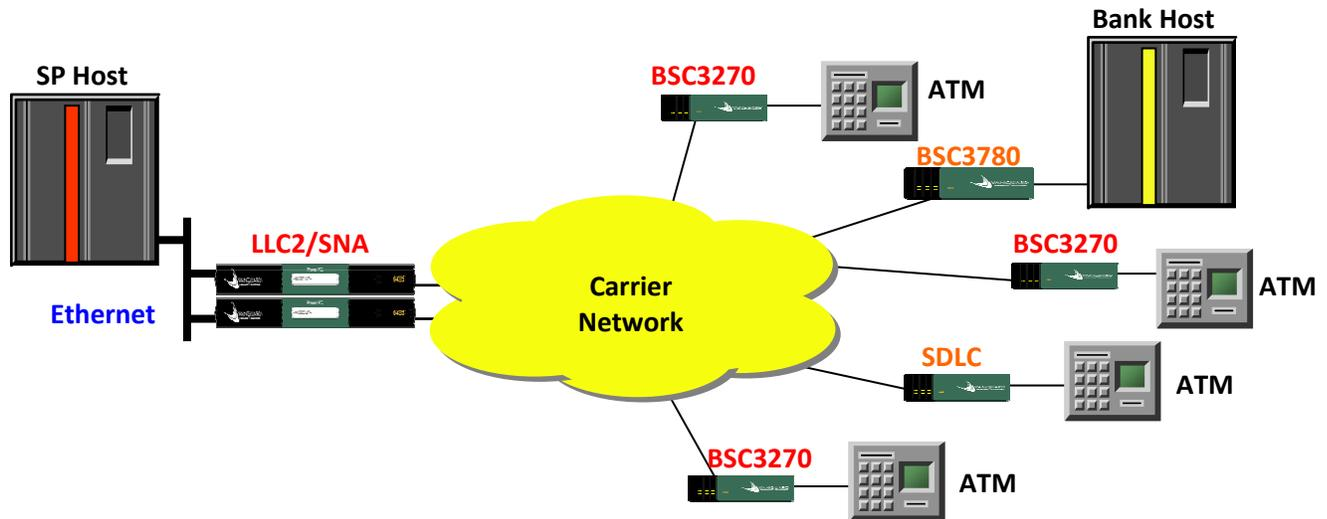
**BSC3270 ATMs, SDLC ATMs, and a BSC3780 bank host processor are all terminated on the Service Provider's IBM host via an Ethernet LAN connection. All BSC and SDLC protocols are terminated at the remote locations and only data is passed across the network.**
