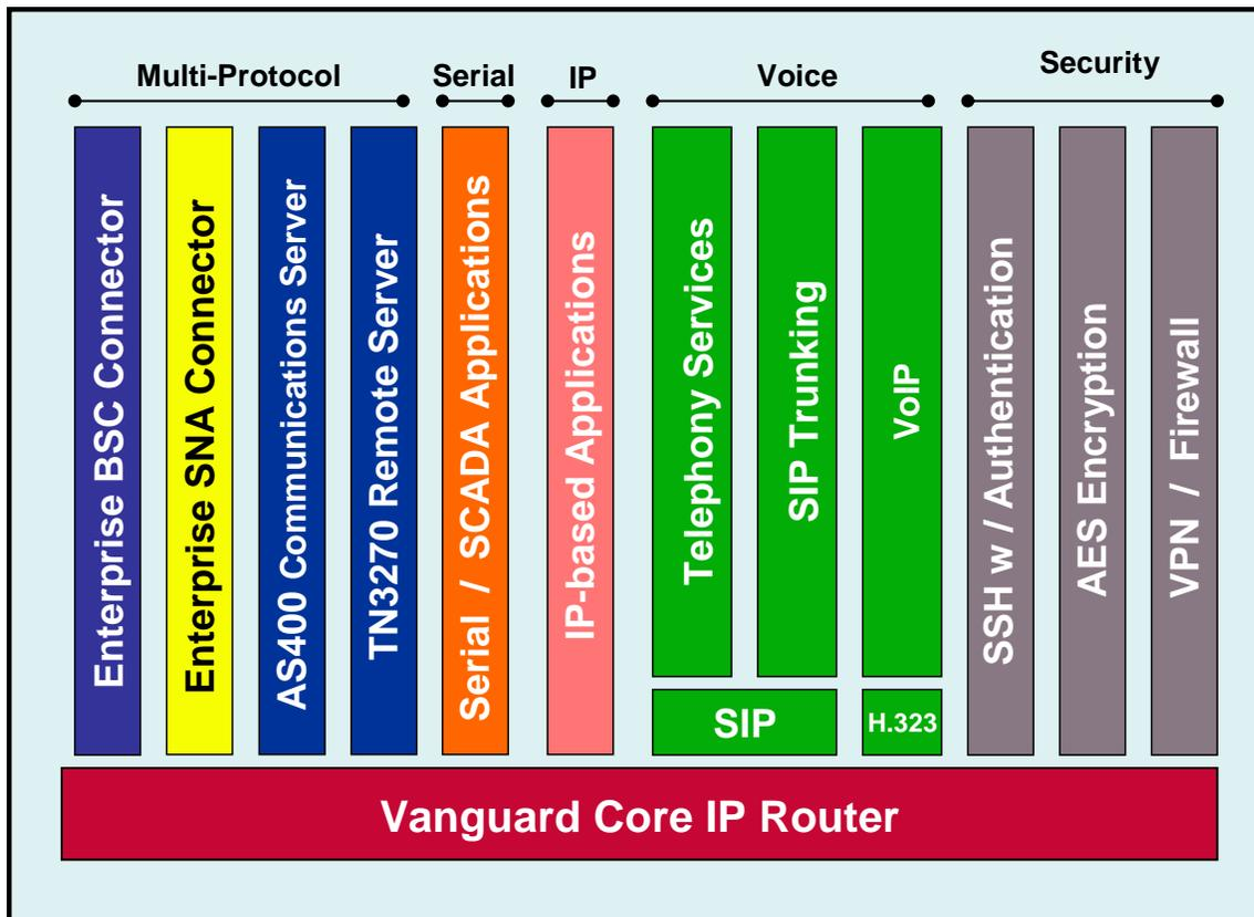
Enterprise SNA Connector is one of the many applications offered in the ApplicationsWare suite that operate on the Vanguard IP Router base platform. All applications can be run across a single wide area network environment.
