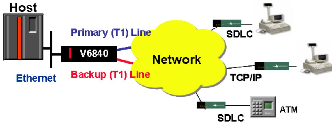
**SDLC ATMs, teller terminals and POS controllers are all connected to the IBM host via a Ethernet LAN connection. All SDLC protocols are terminated at the remote locations and only data is passed across the network.**
