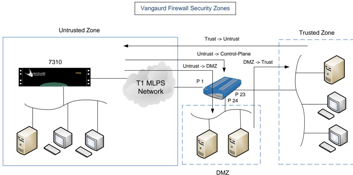
The Demilitarized Zone (DMZ) provides external users a controlled access to resources. The Control-Plane controls any incoming data directed to internal interfaces in the Vanguard Networks Router itself.
